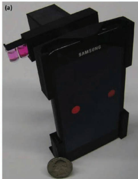
Colorimetric smartphone based platform for allergens Lab Chip, 2013, 13, 636–640
