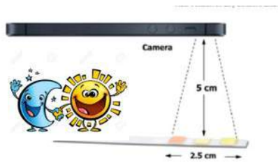
Fig. 1. Quantifying colorimetric tests through a smartphone reader. The smartphone captures and processes the image of the test zones, reducing time and errors related to visual inspection of the color reference chart.
